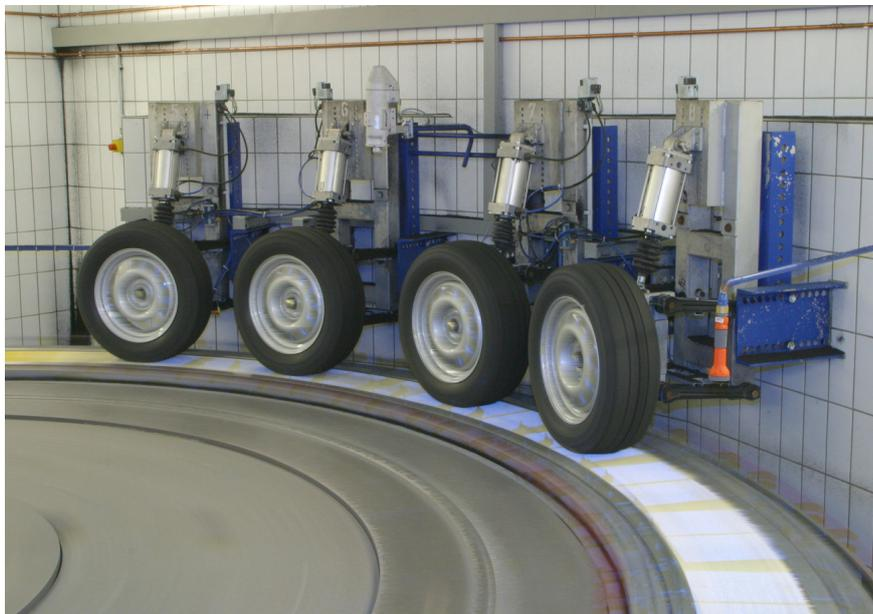
The turntable road-marking test system of the Federal Highway Research Institute (BAST)
