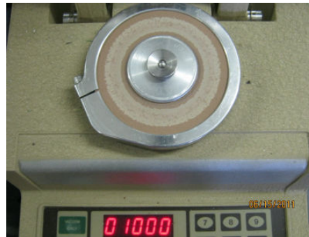
Photos of Taber Abrasion Test at 1,000 cycles, no wear through of coating.
